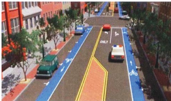
Carlisle, PA Road Diet
