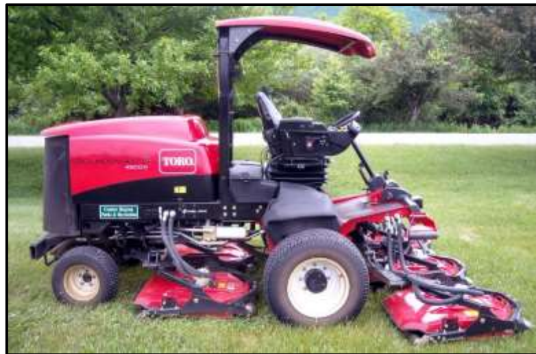
Figure 77. This 2013 CRPR mowing tractor cuts a 10' wide swath on sportfields across the Centre Region.
